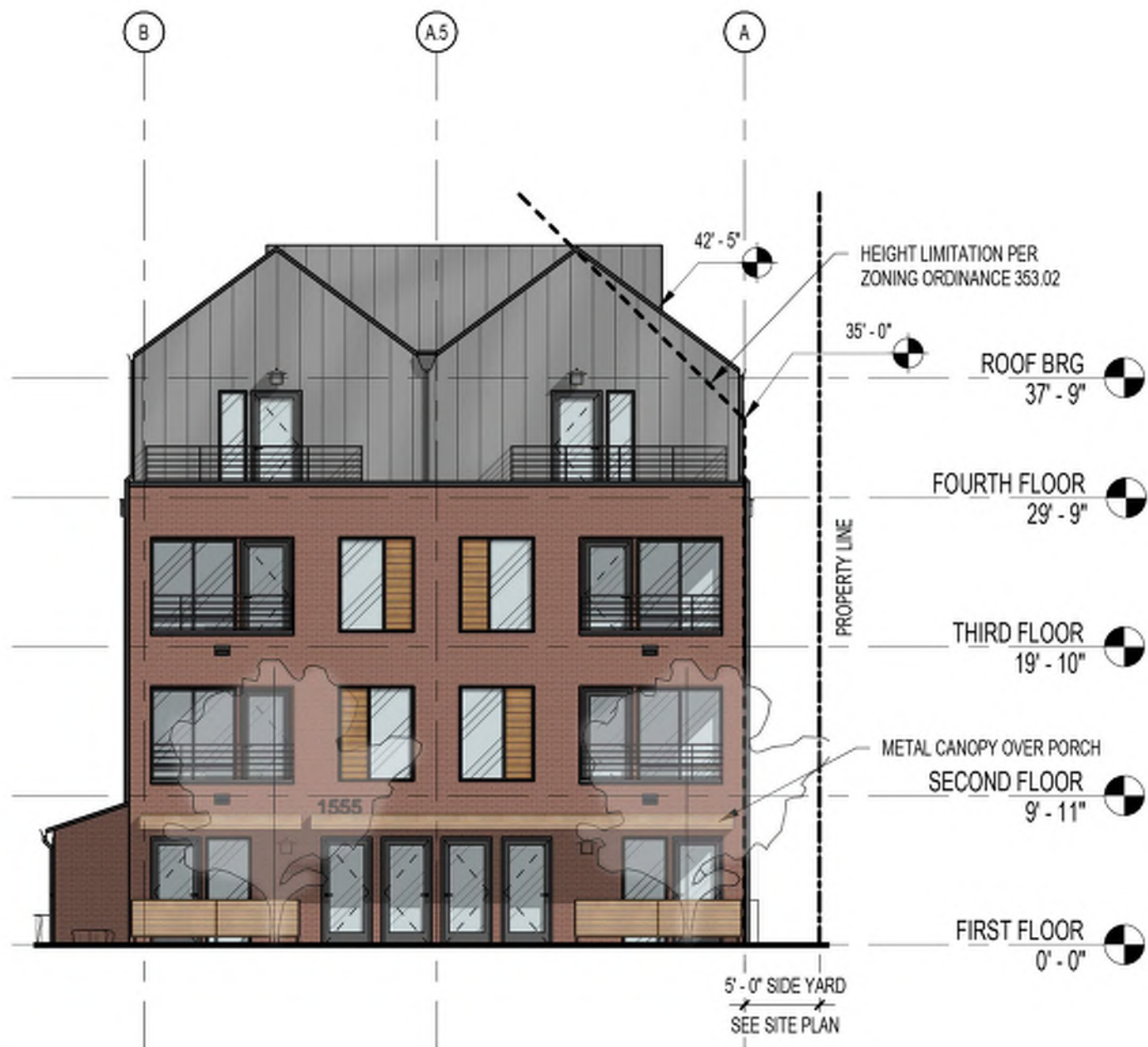
1 WEST EXTERIOR ELEVATION - BLDG A 3/32" = 1'-0"
