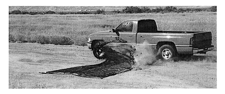
CAPABLE OF STOPPING VEHICLES RANGING FROM SMALL CARS THROUGH TO 10 TON LORRIES
